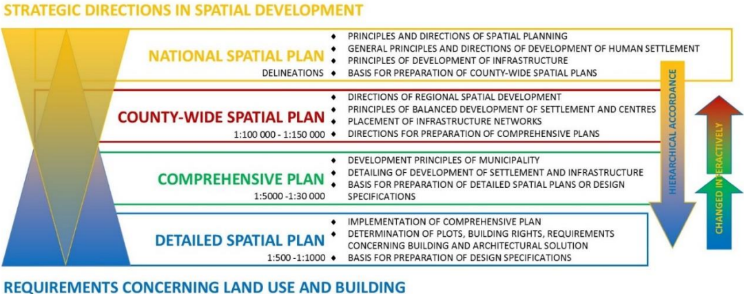
A general structure of planning system in Estonia
