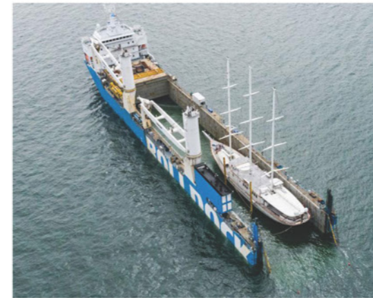
Example of an open dock vessel (source: CONCEPTONTWERP HUB IN HET MARIPARK, Marin )
