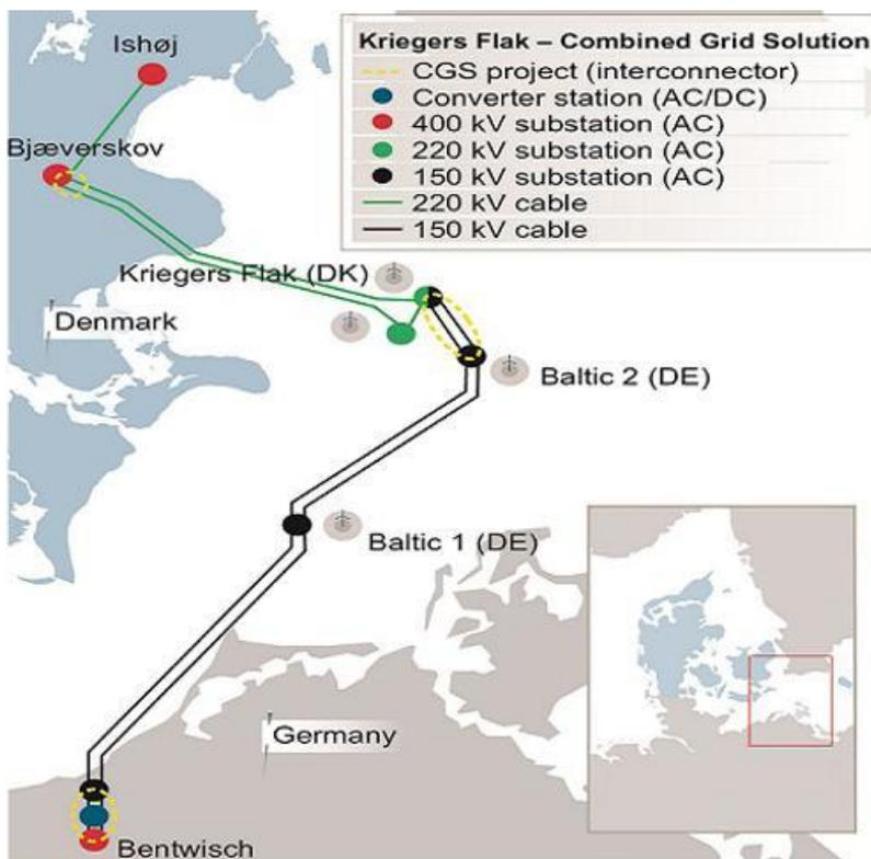
Figure 9: Kriegers Flak CGS between Germany and Denmark, Source: Energinet.dk (<http://www.energinet.dk>)
