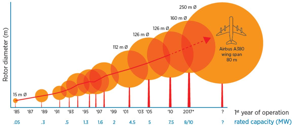
Figure 34: Progression of wind turbine sizes and their rated energy output (MW) up to 2017 and outlook (Lako & Koyama, 2016)
