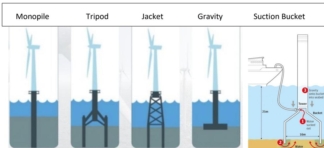
Figure 36: Different substructures used in offshore wind (Arnoudt & Triest, 2013) (4cOffshore, 2018)
