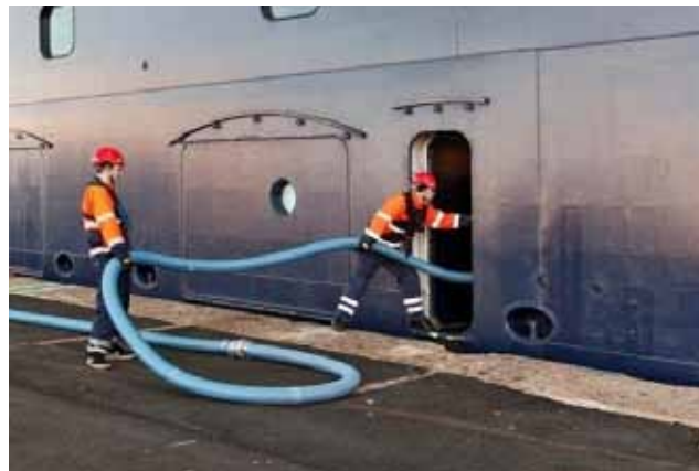
Port Reception Facilities for ship sewage at the Port of Helsinki.
