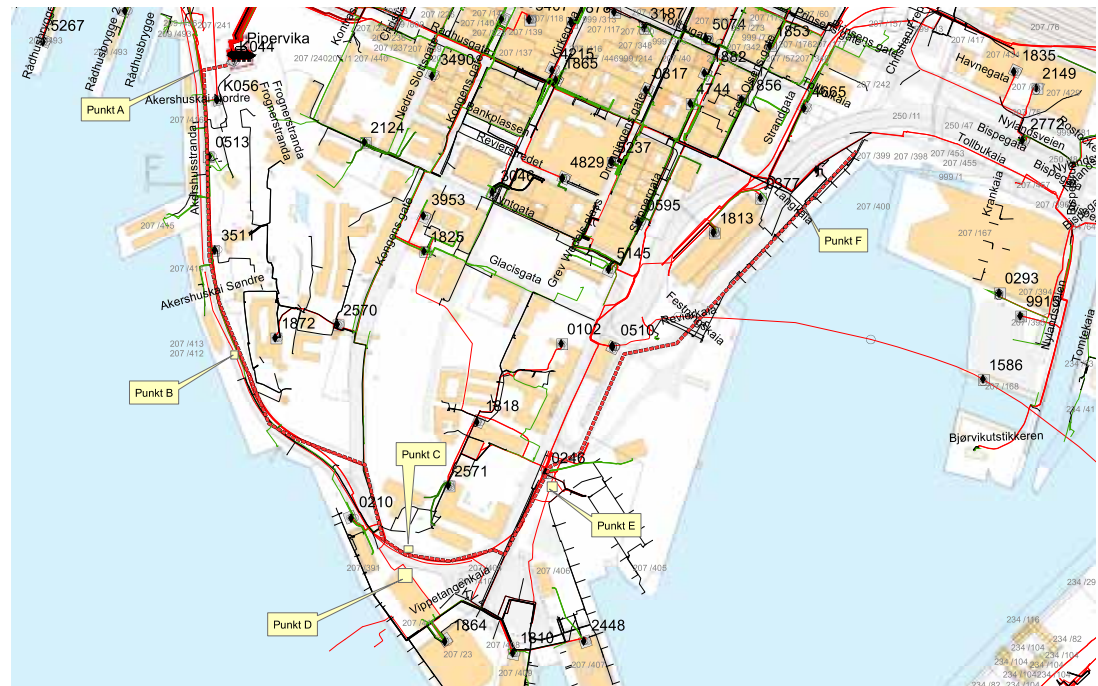
Existing and planned cabling in the Port of Oslo.
