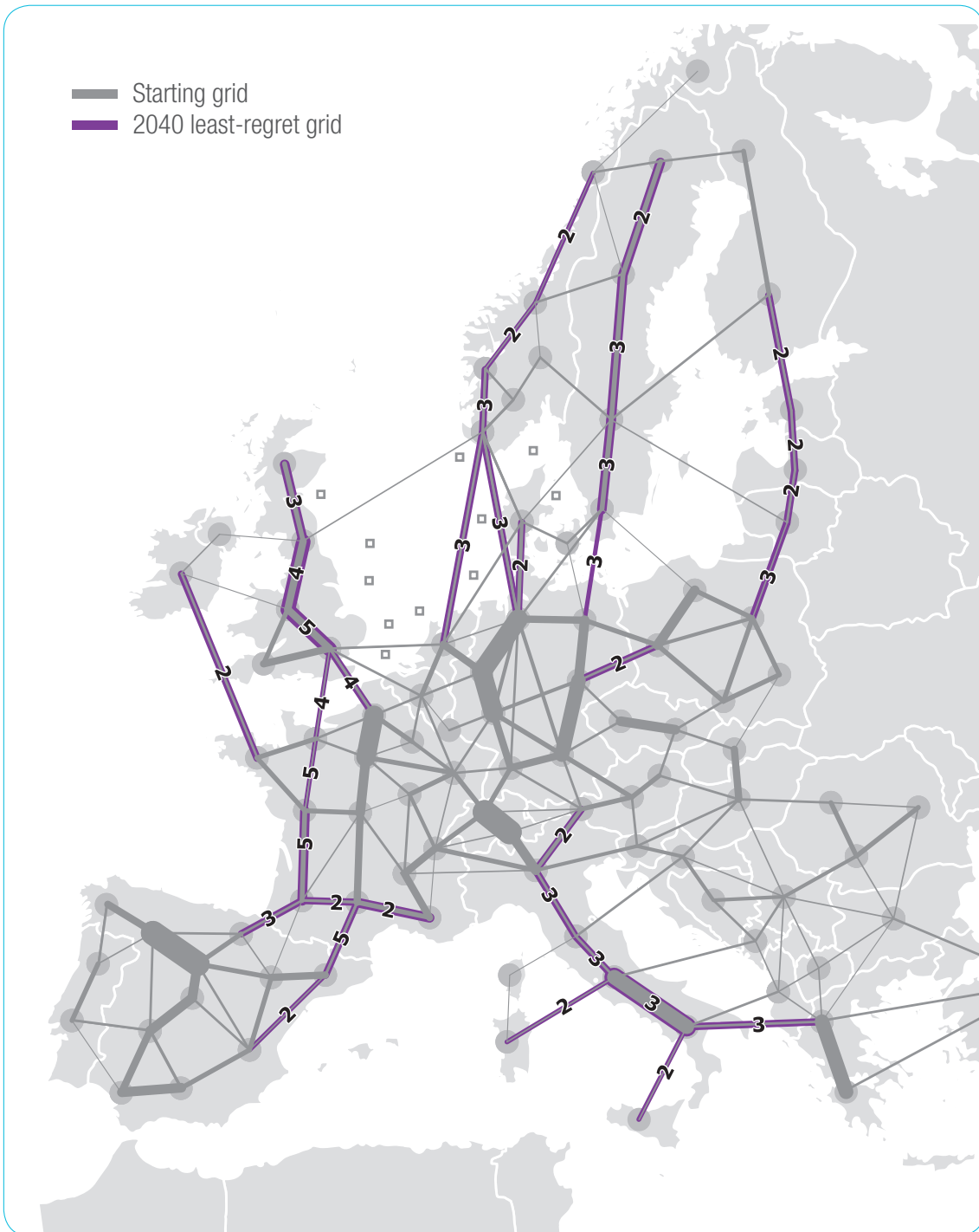
Figure 18: Grid architecture for 2040, robust to the five scenarios (grey: starting grid; purple: reinforcements)
