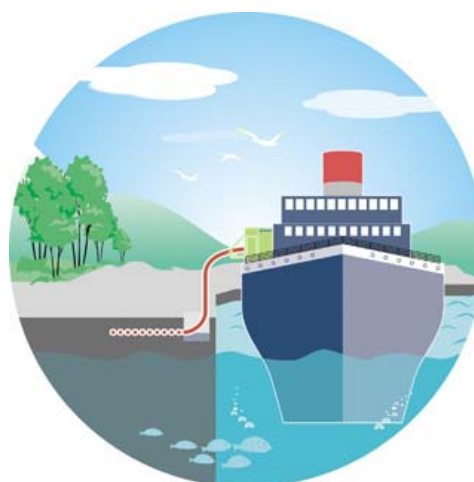
Figure 1: Onshore Power Supply (OPS)
