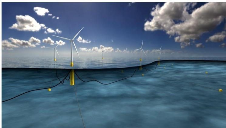
Figure 37: The world's first floating wind farm, Hywind pilot park, 25 km off the coast of Peterhead, Aberdeenshire in Scotland (Source: Equinor/ Statoil<sup>4</sup>).
