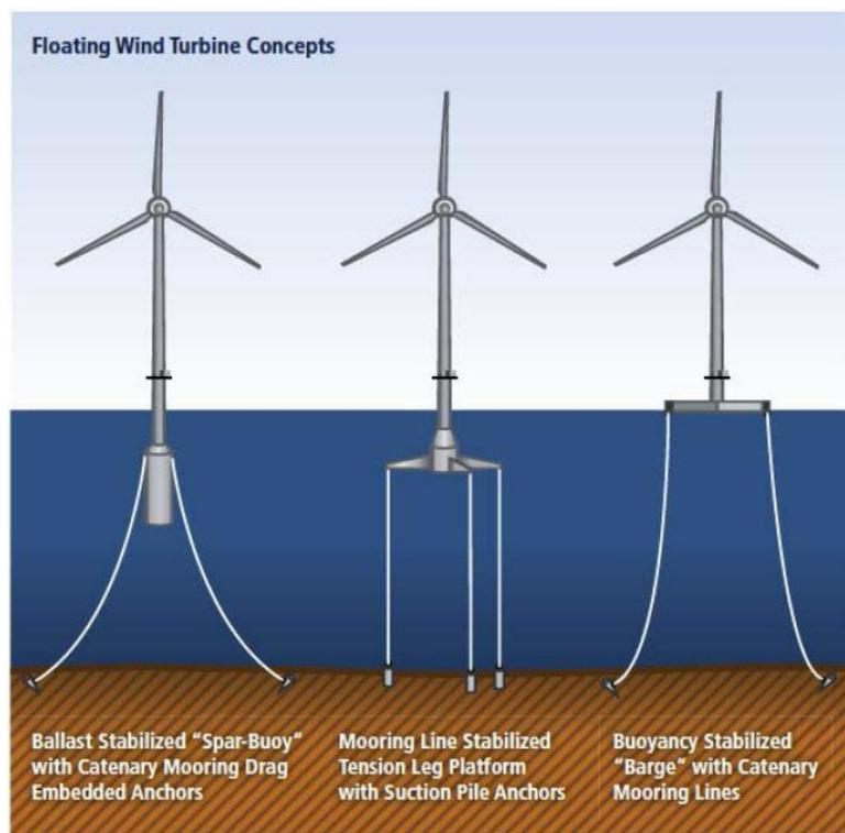
Figure 38: Main technologies for floating offshore wind (Source: Global CCS Institute<sup>5</sup>). Equinors concept builds upon spar buoys concepts that require deep water, while other substructures might work on shallow water as well. Semisubmersible and spar buoy floating substructures are deemed feasible, while the barge and the tension leg platform (TLP) floating substructure concepts are still under development in offshore wind.
