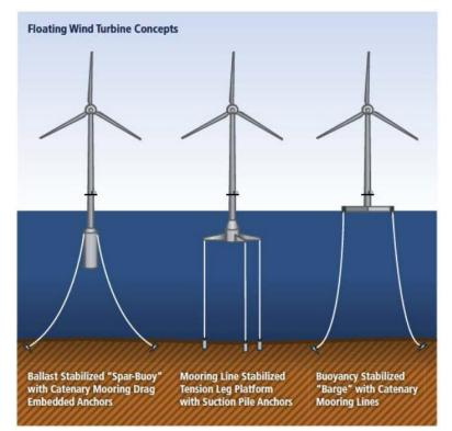
Figure 38: Main technologies for floating offshore wind (Source: Global CCS Institute<sup>5</sup>). Equinors concept builds upon spar buoys concepts that require deep water, while other substructures might work on shallow water as well. Semisubmersible and spar buoy floating substructures are deemed feasible, while the barge and the tension leg platform (TLP) floating substructure concepts are still under development in offshore wind.
