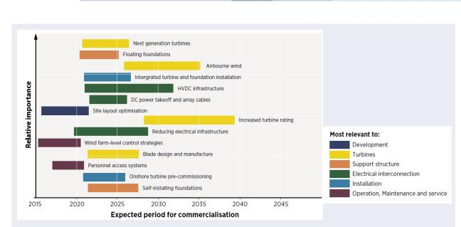
Figure 39: Anticipated timing and importance of innovations in offshore wind technology, 2016-2045, (Freeman, et al., 2016)
