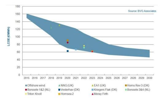
Figure 26: Drop in costs for offshore wind projects based on commissioning date, LCoE (Chamberlain, 2018)
