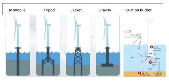
Figure 36: Different substructures used in offshore wind (Arnoudt & Triest, 2013) (4cOffshore, 2018)
