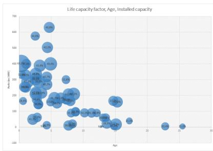
Figure 29: Life capacity factor of wind farms in the UK, Denmark, Belgium and Germany [%], based on data from <u>http://energynumbers.info</u>. Capacity factor compares the name plate rating of a turbine/ park (its maximum power production) with the real production during a certain period of time affected by e.g. lower winds or outages)
