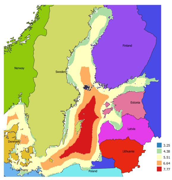
Figure 4: Average wind speeds [m/s, one hour mean] in the Baltic Sea based on numerical simulated data from coastDat
