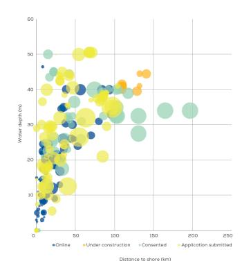
Figure 35: Average water depth, distance to shore of bottom-fixed, offshore wind farms by development status. The size of the bubble indicates the overall capacity of the site (Fraile, Mbistrova, Pineda, & Tardieu, 2018)
