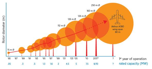
*Figure 34: Progression of wind turbine sizes and their rated energy output (MW) up to 2017 and outlook (Lako & Koyama, 2016)*
